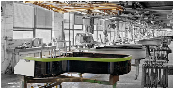
Steinway Precedent 5 Fitting the Braces and Plate
