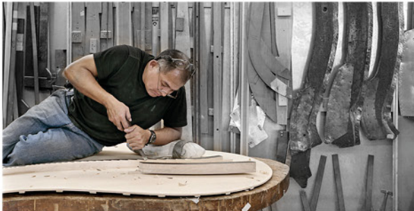
Steinway Precedent 8 Bellyman Installation
