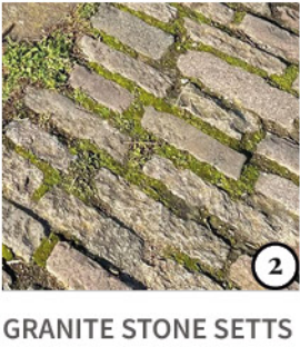
GRANITE STONE SETTS Spec.: Naturally Weathered Colour: Blue-Grey-Pink Dim.: 100 x 100 x 200–300 mm Mortar: 10–15 mm
